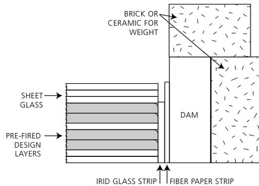
CROSS-SECTION OF DOUBLE-FIRE STACK
