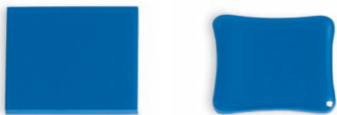
Figure 3: One, 1/8" (3mm) layer fired to 1500°F (816°C). Notice how the edges pull in.
