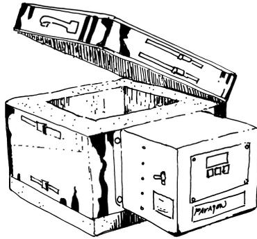
The Caldera is rated at 120 volts and 14 amps. The entire unit stands about 10.5" high and is 13" by 21" with the control box. To be used as a Vitrigraph, it is set on top of a panel of 1" thick rigidized fiberboard that replaces the bottom of the kiln. This 12" square panel has had a 2.5" diameter circle cut out of its center. The entire unit is mounted overhead either to a wall or on a sturdy ladder-like structure. Our Vitrigraph is mounted with
