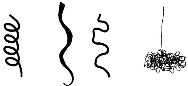
**Hand pulling.** Many types of lines require only handwork (gloved, of course!). If the glass is viscous enough you can pull it at intervals to create stringers of fluctuating thickness. At these low temperatures the glass can also be pulled into curves. At very high temperatures when the stream is extremely thin and fast-moving you can make delicate bird's nest shapes and meshed globs by allowing the stream to "free fall."
