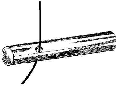
**Pipes.** Stringers in the shape of spring-like coils are made using a 1" diameter steel pipe. Ours is 15" long with 1/2" holes drilled through the wall about 1" from the pipe's end. Pull the glass stream through the drilled holes. As the glass flows, twirl it around the pipe and then cut or break it at the end of the pipe.
