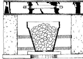
Within the heating chamber a pair of mullite clay strips (sawn up kiln shelves) are bridged across the center opening in the fiberboard in order to support a clay flowerpot. This pot is about 5" high with a 6" diameter rim. Avoid pots with hairline (or larger) cracks as these will widen as they reach molten glass temperatures. In our experience Italian pots seemed more durable than those from Mexico.
